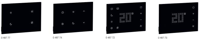
Touch devices for an intuitive and easy use of different rooms functions These devices have to be associated with room controllers IP/Bacnet Cat.No 0 484 08/12 or IP scenario module Cat.No BT-MH201 Possibility to customize touch control using configurator on Legrand website: icon, color, hotel logo, mounting support, etc Connection to a 27 V BUS power
