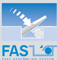
Slot base wires of the tray into the cantilever arm and bend tabs with screwdriver to secure, as shown in the FAS diagram above
