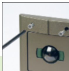
1 Remove the 4 screws using the appropriate tool
